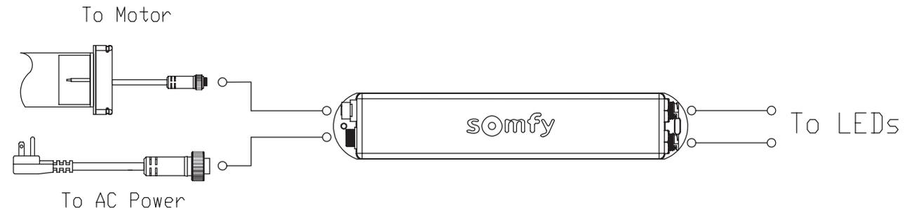
**Example 1:** Utilizing the Sunea® motor the receiver is plugged into the motor and both are powered from the same source via Sunea® power cord. The field installable motor plug allows the same configuration with other motors.
