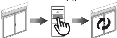
4. Press and hold **DOWN** button, run motor to desired **DOWN** limit position.
