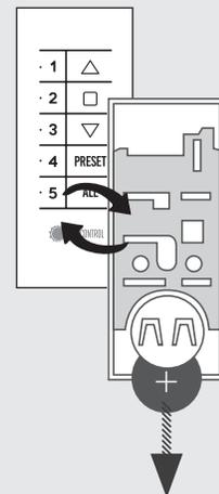
Insert the new battery respecting the correct polarity.
