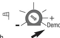
**The change of setting "In" or "Out" of the Demo Mode is confirmed with a brief Jog of the motor. This function can be used to confirm the sensor is communicating with the motor's receiver.**
