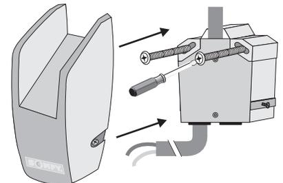
5. Attach the sensor to the wall.
